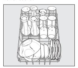
The lower basket glassware insert is designed for washing tall glasses. Tall glasses are held securely by the vertical supports.
